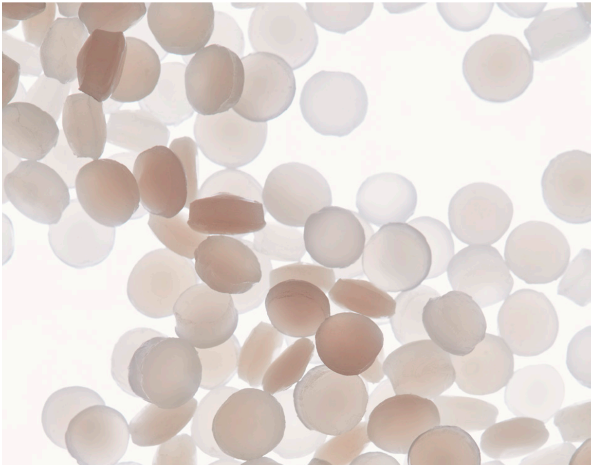
Plastic pellets produced from recycled material at Stena Nordic Recycling Center.
