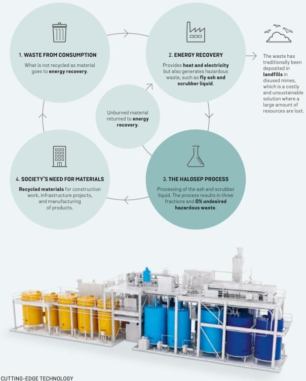
A 3D model of a typical HaloSep plant.
