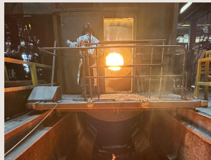
Technician in protective clothing controls the process where the purified slag is heated to 1,600 degrees. Photo: Swerim
