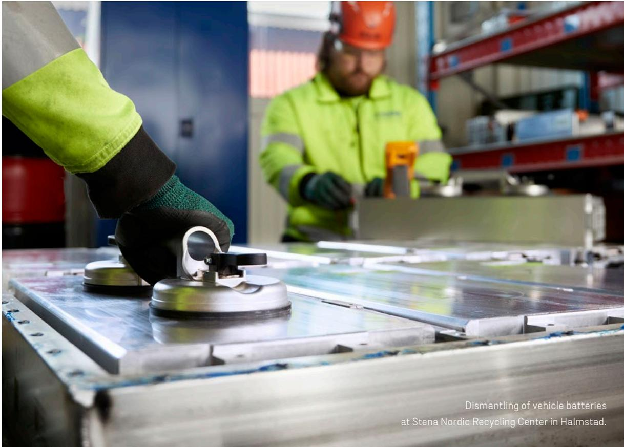
Dismantling of vehicle batteries
