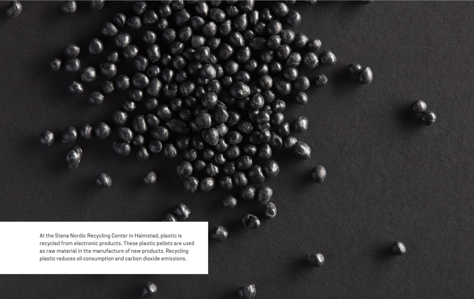
At the Stena Nordic Recycling Center in Halmstad, plastic is recycled from electronic products. These plastic pellets are used as raw material in the manufacture of new products. Recycling plastic reduces oil consumption and carbon dioxide emissions.
