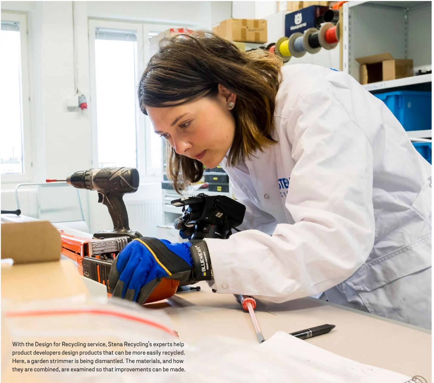
With the Design for Recycling service, Stena Recycling's experts help product developers design products that can be more easily recycled. Here, a garden strimmer is being dismantled. The materials, and how they are combined, are examined so that improvements can be made.
