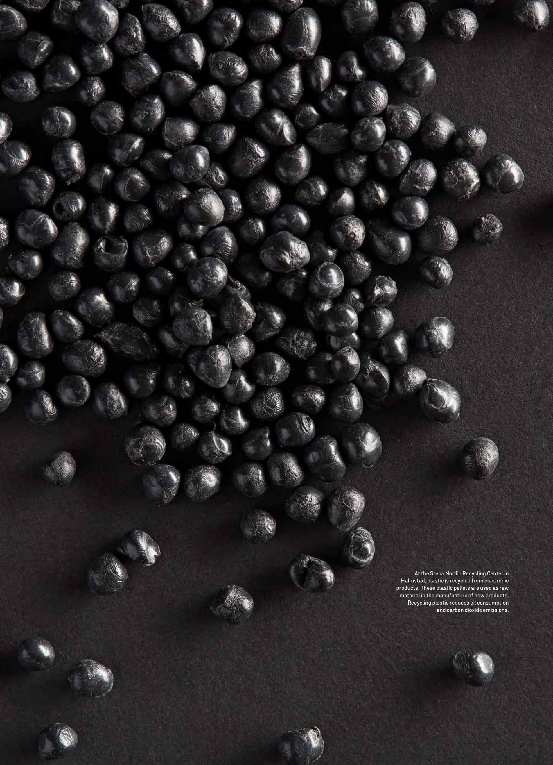
At the Stena Nordic Recycling Center in Halmstad, plastic is recycled from electronic products. These plastic pellets are used as raw material in the manufacture of new products. Recycling plastic reduces oil consumption and carbon dioxide emissions.
