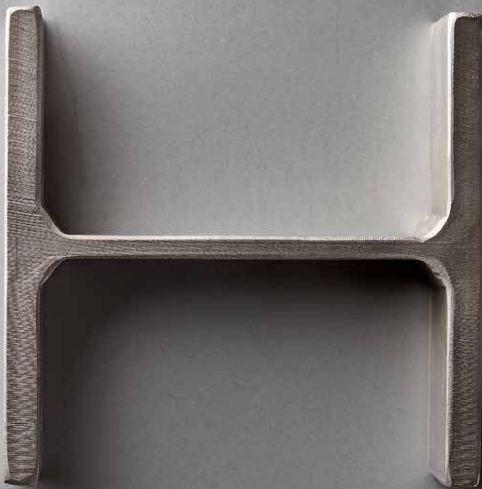
Cross section of a HEA beam, one of the products in Stena Stål's wide range.
