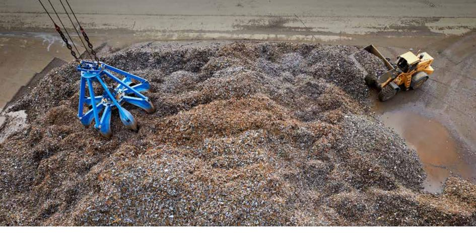
Shredded ferrous scrap, to be exported to a steel mill in Turkey, being loaded on a ship in the port of Halmstad.
