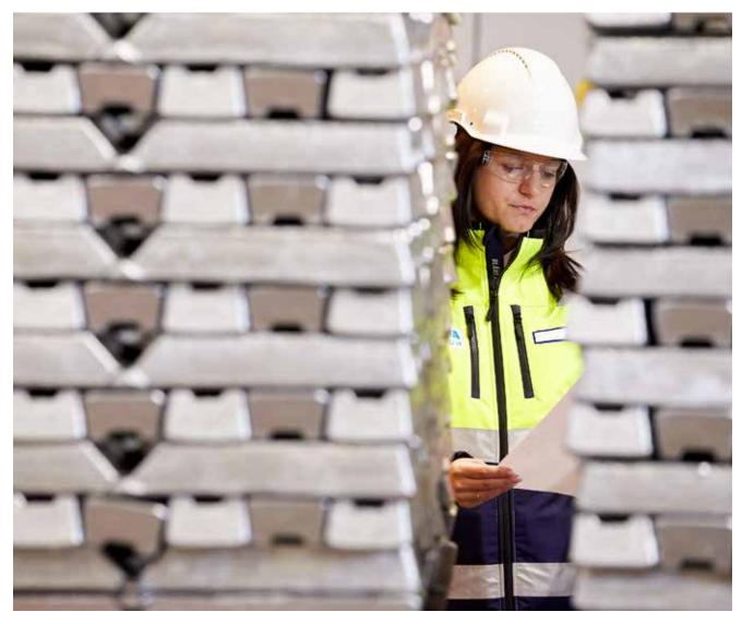
Major environmental benefits in aluminium recycling. Producing aluminium from virgin raw material, in the form of bauxite, consumes large amounts of energy. Aluminium produced by recycling can reduce energy consumption by around 95 percent. In principle, aluminium is infinitely recyclable without losing any of its properties. Aura Popescu is responsible for indirect purchasing, here pictured at Stena Aluminium's warehouse.
